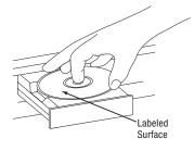
To retract the drawer back into the player after loading a disc, press the Open/Close button **3 (b**). When the drawer is closed the display will indicate the total number of tracks on the disc and the total running time of the disc.
