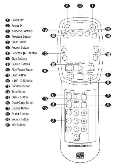
Power Off: Press this button to put the unit in the Standby mode.
