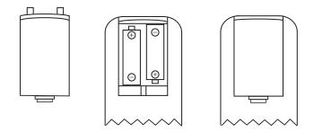
Install two AA batteries by turning the remote over so that you are holding the bottom side up. Press lightly on the embossed arrow on the cover and gently slide the cover toward you in the direction of the arrow. Insert the batteries inside the compartment, being careful to follow the + and - polarity indications at the bottom of the compartment. Replace the cover by placing it on the remote and sliding it back toward the top of the remote.
